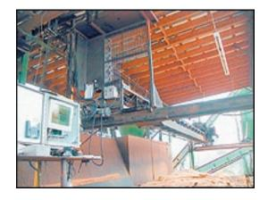
Streamline your mill with our computerized setworks. Increase efficiency and get rid of the headache of doing the math, let the computer do it! With one touch of a button, the saw head will move to a preset distance. You no longer have to manually make the usual fine adjustments required when doing it by eye.
